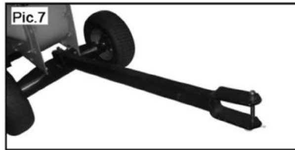
Pic.7 Attaching the tow rod
